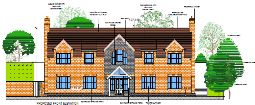
Proposed front elevation of the replacement dwelling
